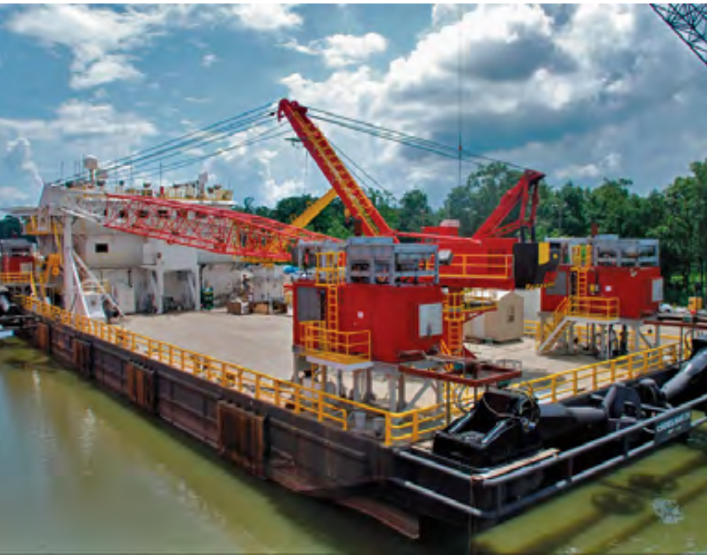
PDPS installed on the Crossmar 21 - a 260 ft (80 m) offshore construction barge. Its DPS-3 system uses four 1000 HP (750 kW) thrusters.
