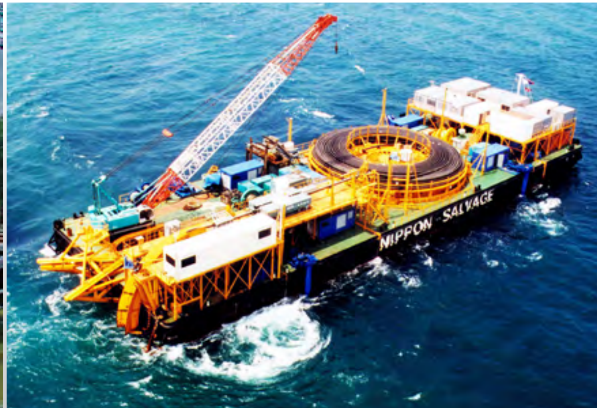
PDPS installed on the 270 x 85 x 17 ft (82 x 25 x 5 m) reel pipelay barge owned by Nippon Salvage. The system allows subsea pipelay installation many times faster than can be done with an anchor moored barge. Uses four 500 HP (380 kW) azimuth thrusters.
