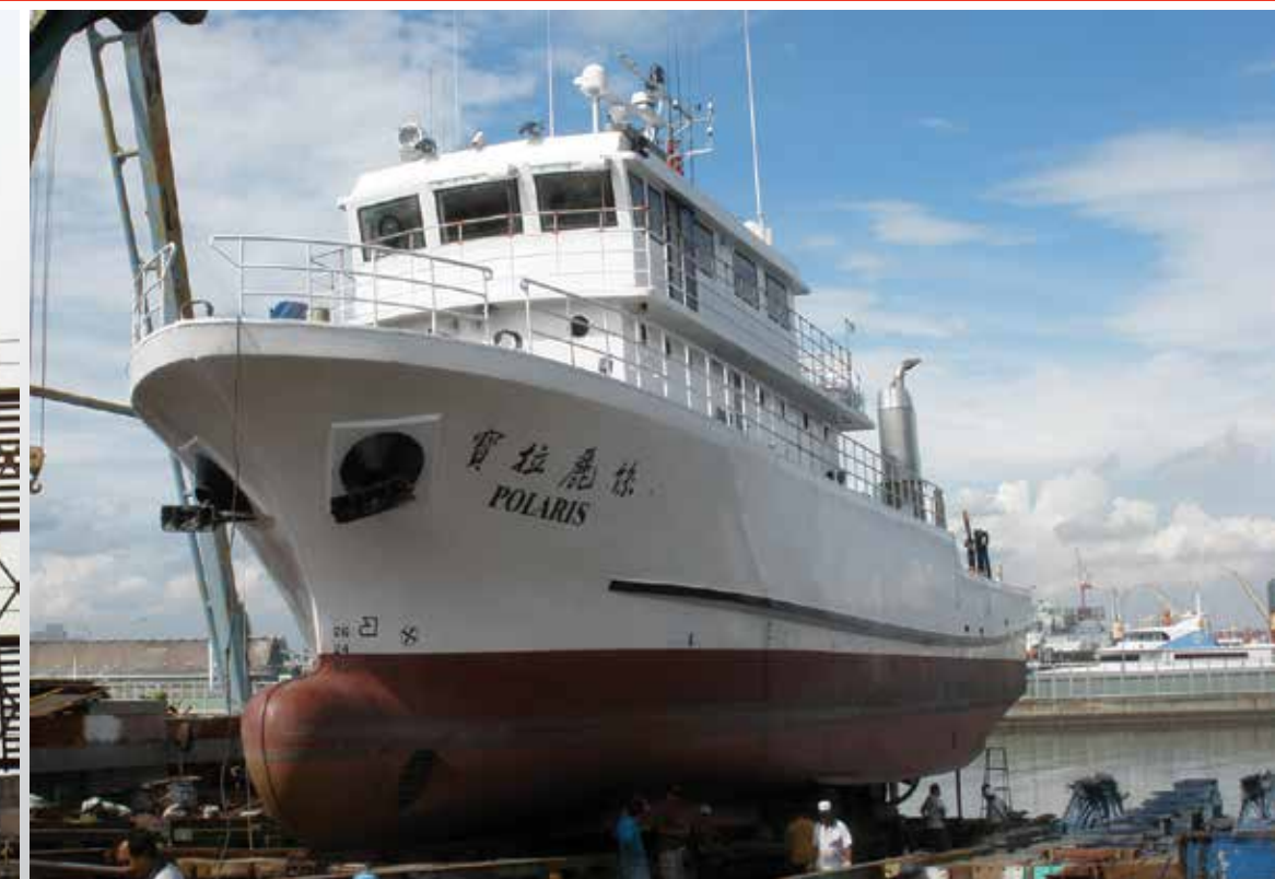
200 HP (150 kW) model 30TT200 hydraulic tunnel thruster installed on the research vessel Polaris along with two hydraulic azimuth thrusters model TH300N.
