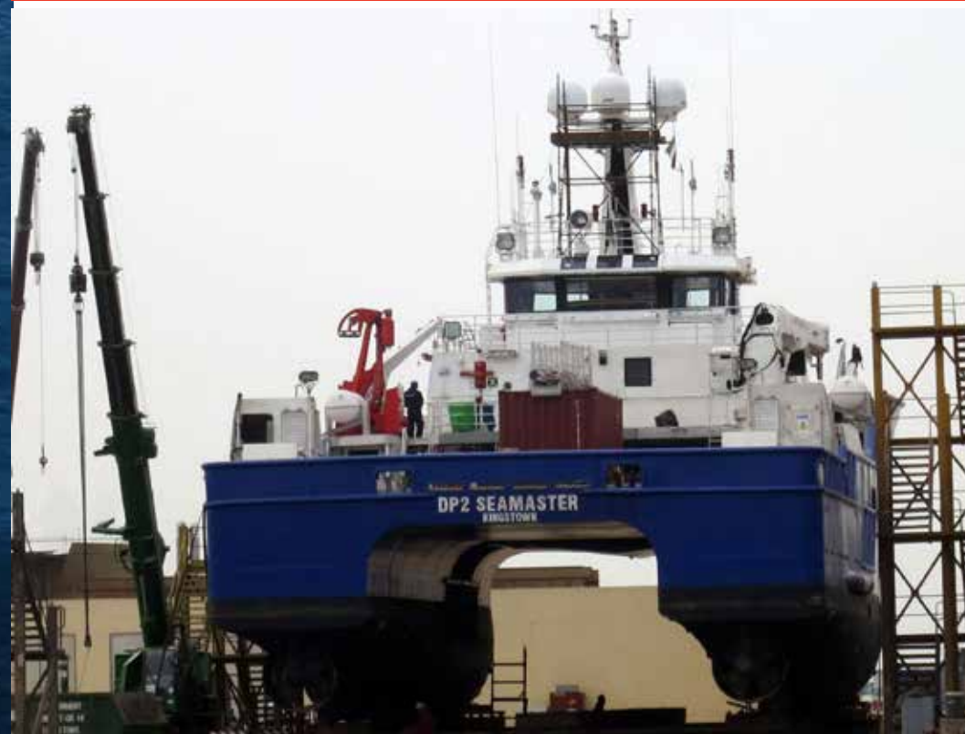
Four 250 HP (185 kW) aluminum hydraulic tunnel thrusters model 36TT250-AL installed on Seaworks' diving support vessel "Seamaster". For main propulsion, the vessel uses two Thrustmaster azimuth thrusters model TH1000MZ of 1000HP (750kW) each.
