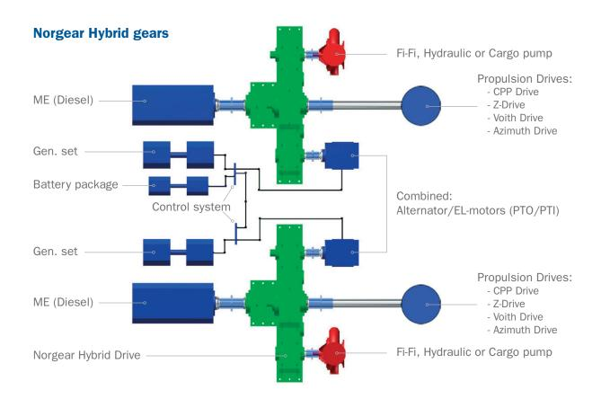
The Norgear Hybrid gears are available with and without auxiliary drives for Fi-Fi, Hydraulic and cargo pump drives. Built in multidisc hydraulic clutches with soft engagement are standard.
